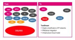
The network for which running code is in place at DTAG's subsidiary <u>Telekom Croatia</u> (500 customers according to Axel Clauberg at DTAG) is based on an IPv6-only network; IPv4 is a *"service" realized via what Löthberg said were "keyed IPv6 tunnels" and what Telekom Labs described as a "special lightweight 4over6" tunneling procedure. IPv6 will be the language of the new network, and all non-IP-traffic is forwarded via Carrier Ethernet.*
